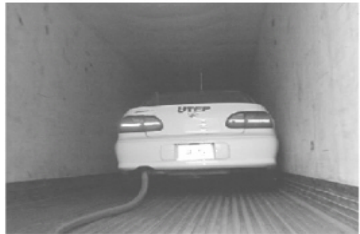
Figure 3. EVC vehicle inside refrigerated trailer for cold start testing.
