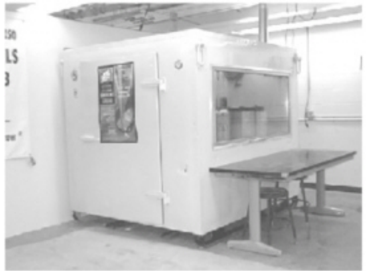
Figure 2. Photograph of the Engine Cold Start Test Facility.
